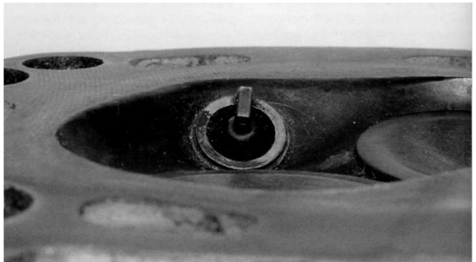
The spark plug electrode is proud of the gasket face on this cylinder head.
