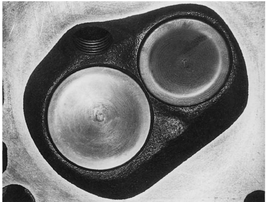
44.4mm Inlet valve and 38mm exhaust valve fitted to a Pinto combustion chamber.
