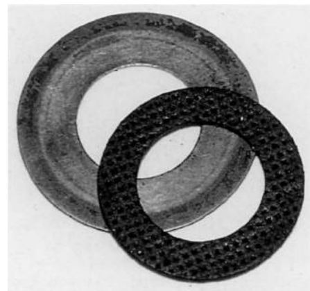
Shims used to control spindle endfloat.
