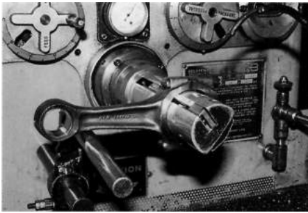
Connecting rod bearing tunnel being honed.
