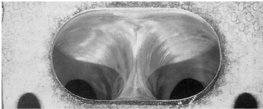
Another view of the completed exhaust port viewed from the manifold end.
