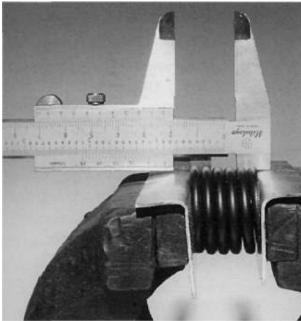
Valve spring compressed between vice jaws and vernier caliper being used to measure the distance between the jaws.
