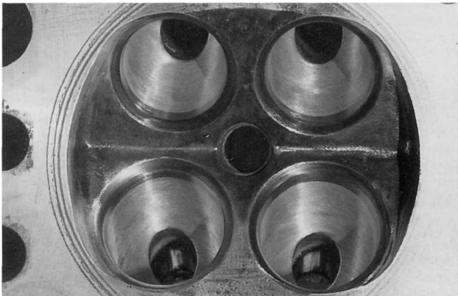
Completed exhaust and Inlet ports viewed from the combustion chamber.
