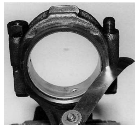
Cap 'sprung' by bearing crush. Feeler gauges inserted between the cap and rod should reveal a 0.1-0.15mm/0.004-0.006in gap.
