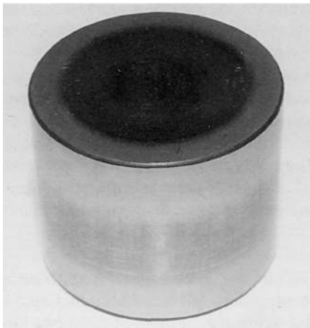
Face of solid lifter for Sierra Cosworth engines with standard length valves.
