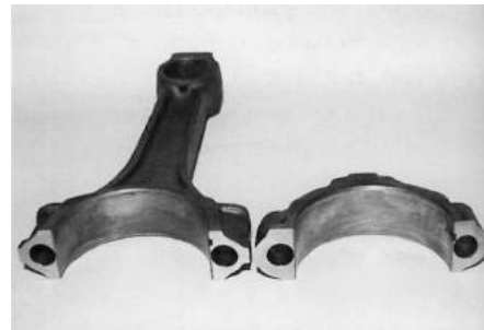
Cap and rod mating faces which have had material removed.
