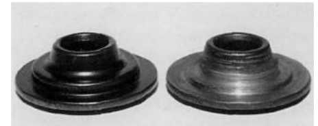
Standard valve retainer (left) and machined down version (right).
