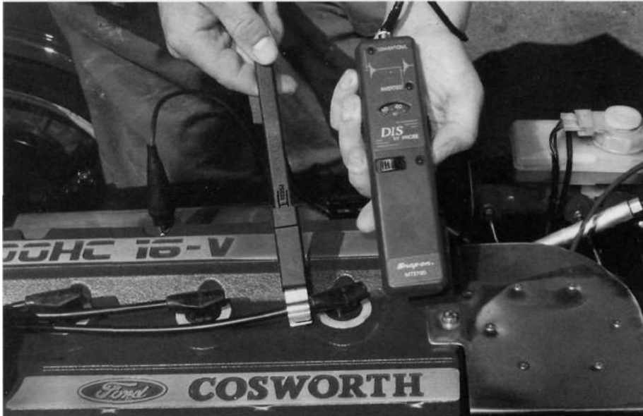
Gunson 'Flashtest' device (top) and Snap-on Tools inductance pick-up device (above) both being used to check voltage at the sparkplug end of an HT wire on a Sierra Cosworth-headed Pinto engine.
