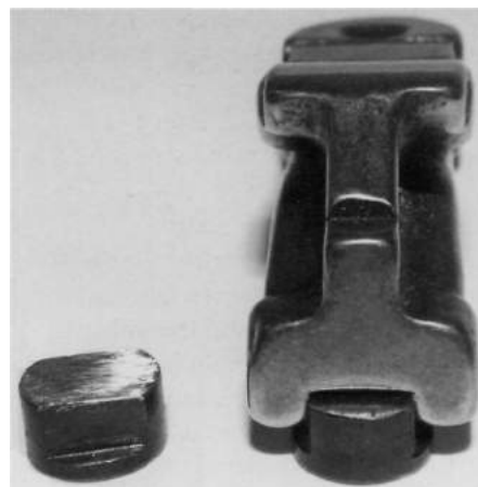
Right. Lash cap fitted into the slot of a rocker just as it would be in an assembled head. Left. This lash cap has been turned 90 degrees to show side machining.
