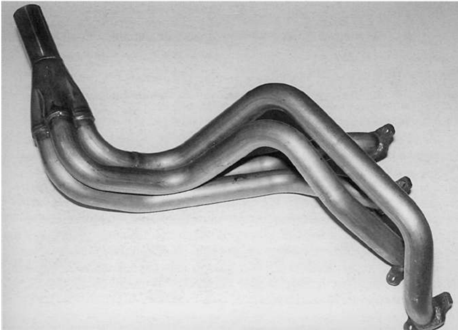
Four into one exhaust system with 42mm/1.625in primary pipes and a 51mm/2in main pipe. The primary pipe lengths are all different!
