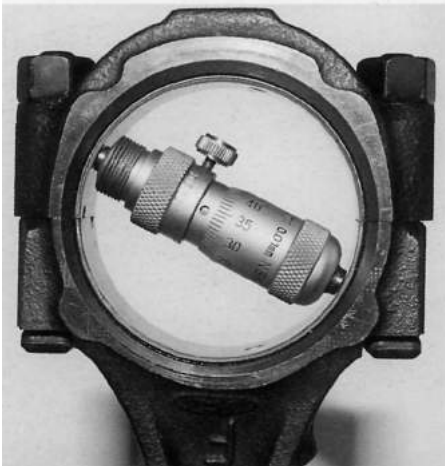
Connecting rod bearing internal diameter being measured in the vertical plane and at 70 degrees to the right and left of vertical.
