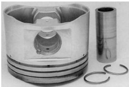
Natural aspiration Cosworth piston, piston pin and wire circlips.
