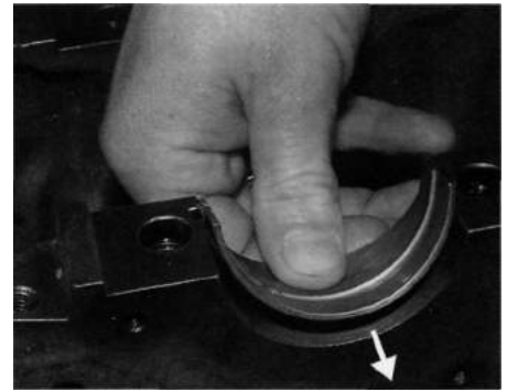
The easiest way to remove a shell is to push it with your thumb in the direction arrowed.
