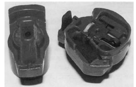
Standard distributor rotor on the left and governor rotor on right.
