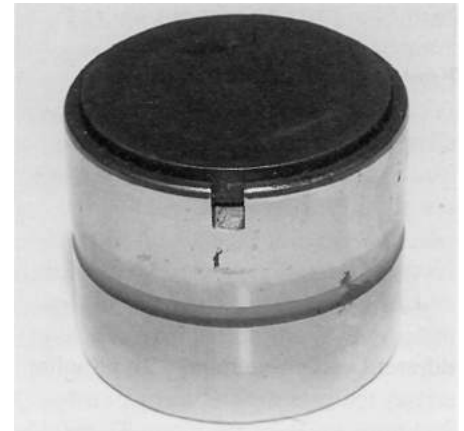
Escort diesel follower with adjustment shim in place.
