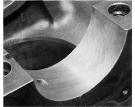
Main bearing tunnel bore surface as machined by the FoMoCo. Nothing less than this finish will do.
