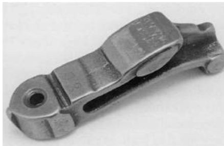
Long pad rocker which has the pad nearer the pivot compared to a standard rocker.
