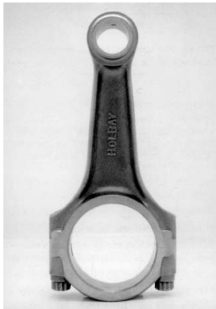
Holbay's 'H' section forged connecting rod.
