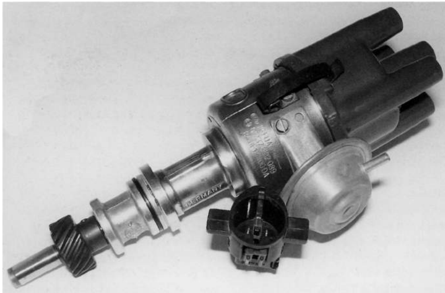
Bosch distributor ('electronic' type), cap and rotor .
