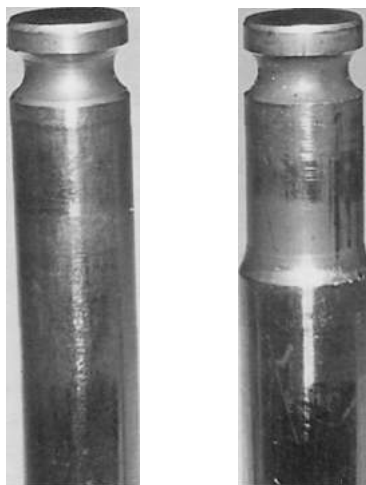
Valve stem keeper groove detail.
