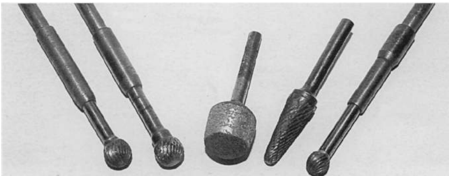
A selection of carbide tools and grinding stone used for porting work.
