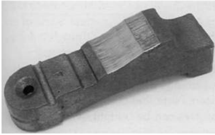
Excessively worn rocker pad as the result of bad geometry.
