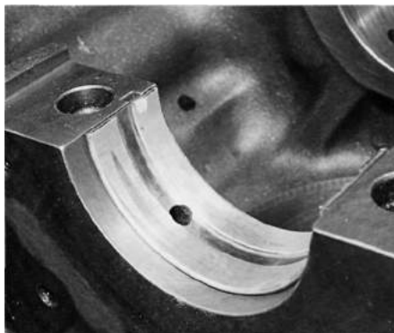
Shell correctly positioned in the block with the ends at equal heights.
