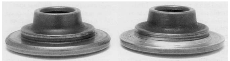
Standard spring retainer on the left and a turned down one on the right. Difference in thickness is 1.25mm/0.049in.
