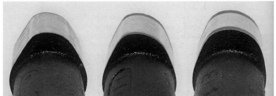
Lobe profile comparison - standard camshaft profile (left), 285 degree high lift camshaft (centre) and 312 degree race camshaft (right).
