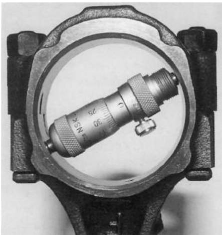
Connecting rod bearing tunnel being measured in the vertical plane and at 70 degrees to the left and right of vertical plane.
