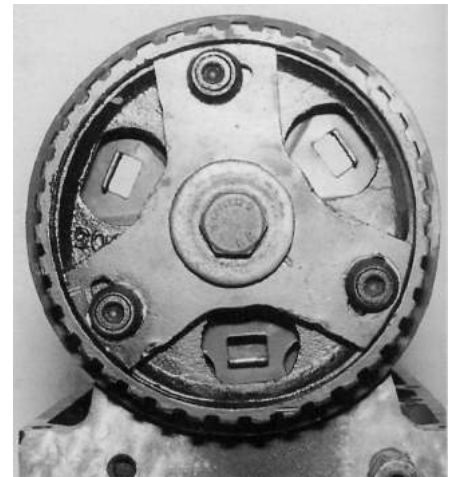
Adjustable ('vernier') camshaft sprocket/wheel.
