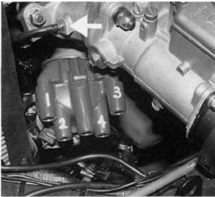
Bosch Peugeot-type distributor cap with horizontal HT terminals. Note vacuum take-off (arrowed) in manifold for vacuum advancesystem.
