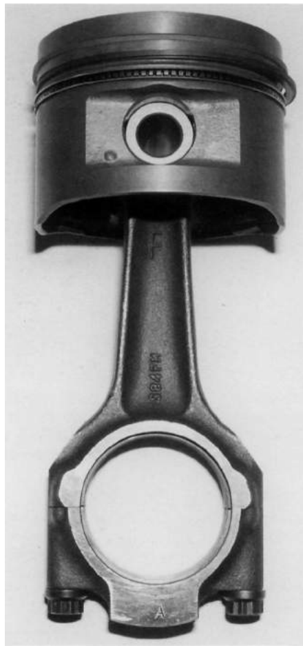
Kolbens Schmidt piston and Fiesta 1600 diesel connecting rod assembly, note the Cosworth connecting rod bolts (a good move).
