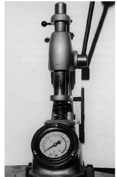
Valve spring pressure testing machine.
