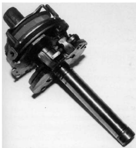
Distributor spindle and cam plate as a unit.
