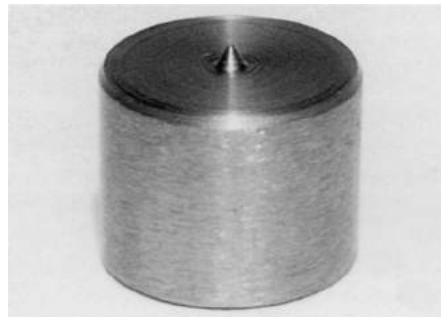
The special spotting punch made to mark the back of the flywheel - the punch must be hardened.
