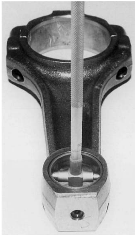
Small end/piston pin bush being measured with a telescopic gauge.
