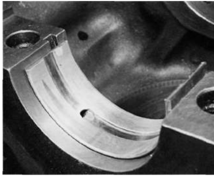
First step in fitting a bearing shell. The location tab is positioned in the machined groove 3mm/0.25in down from the mating surface.
