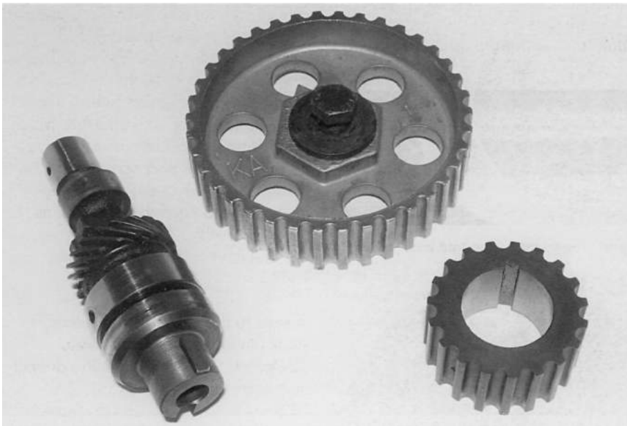
Auxiliary driveshaft (left) nose has been turned down to take a genuine Sierra Cosworth sprocket (right).
