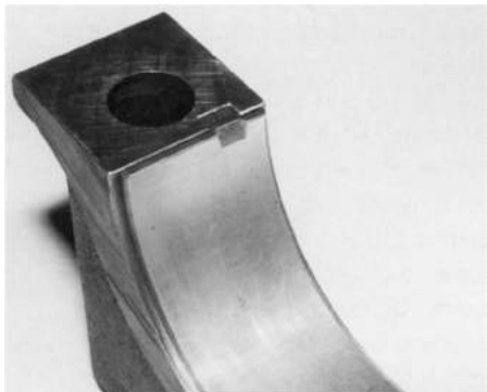
Shell correctly positioned in a cap with the ends at equal heights.
