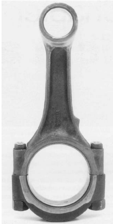
Forged standard connecting rod with lightened small end.
